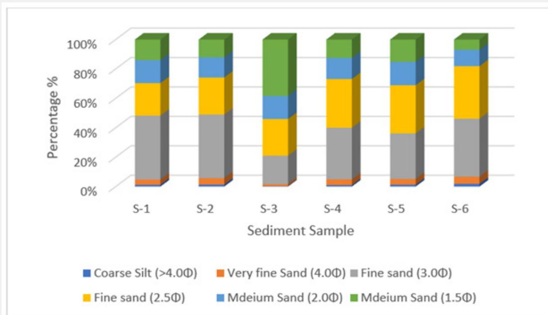
Figure 5: Bar chart shows sediment grain size in percentage where different colors represent percentage of various type of sand.
